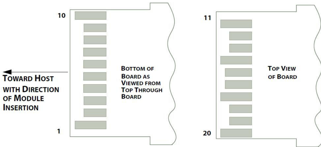
Figure 2 SFP+ module contact assignment
